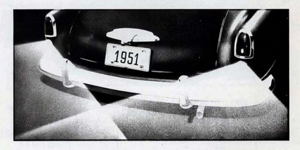
Back-up lights installed in the rear fenders below the tail lamps match the parking lamps.
