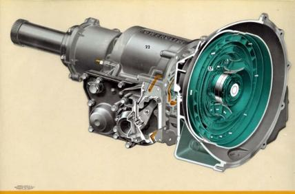
16. Here a section of cover has been removed to expose the modulator control lever. The lever is actuated by a vacuum diaphragm so that changes in engine speed can be bolanced with hydraulic pressure in the POWERGUIDE unit. The purpose of this modulator control is to increase oil pressures when high torque is being transmitted.
