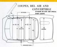
The Bel Air and the Convertible vary in the following dimensions: Bel Air-rear hip room width 52½ inches; front seat shoulder room 53% inches. Convertible-front seat shoulder room 53% inches; rear seat shoulder room 46% inches; rear seat hip room 483% inches.
