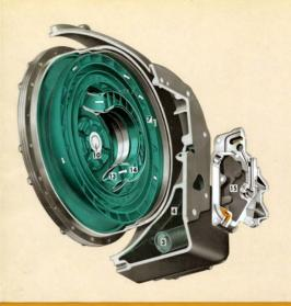
13-14. Cross-section view of the two stators in their "nested-together" position with arrows indicating the direction of all flow. Although these stators remain stationary to multiply torque when necessary, they are to turn with the turbine at high speeds. In this case, POWERGLIDE supplies more speed and less power, even more effectively than the driver could do by shifting a conventional gear transmission into high gear.
