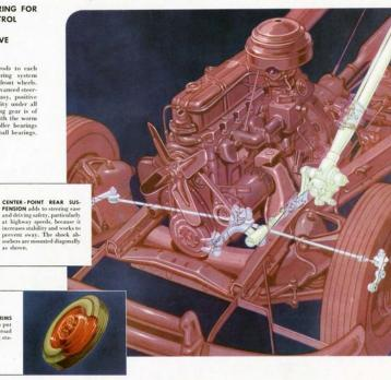
5-INCH WIDE BASE RIMS carrying low-pressure tires put a large soft cushion on the road that adds both to steering stability and riding comfort.
