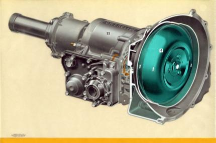
6. External view of trubine or driven member. It is fabricated of high precision steel stompings that are spot-welded and copper brazed to form a single unit. Engine power is transmitted to the turbine by oil. There is no metal to metal contact to cause wear. At peak engine performance, the pump drives oil at the rate of 55 golions (one barrel) per second energize the harbine. Here is flashing power and performance, free from
