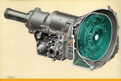
11. Section of modulator control cover. The entire operation of the POWERGUIDE transmission is automatic. When the control lever is moved to positions other than "PARK" corresponding changes within the transmission are accomplished by means of oil pressure and valves. Vacuum from the engine is used in conjunction with oil pressure to effect smooth, siltert and synchronized operations.
