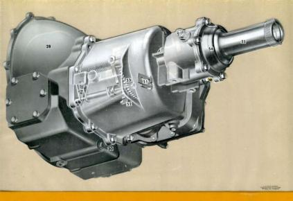
51. This is the mechanical link for the manual valve which operates through the parking lock shaft. When applied, the parking device rigidly locks the transmission to hold the car on the steepest hills or grades.
