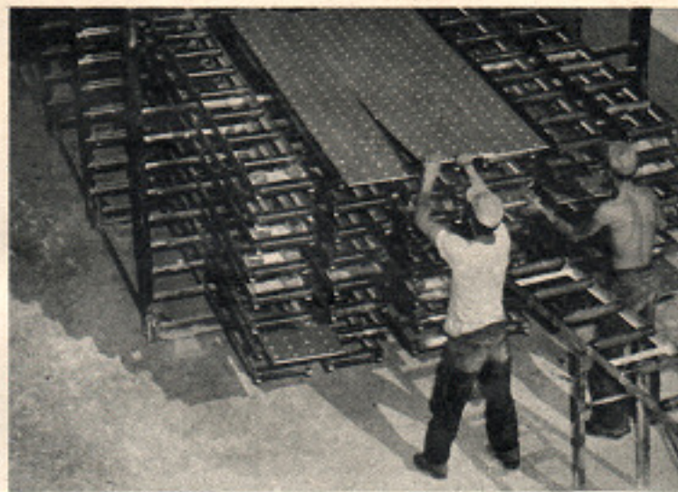
GYPSUM . . . Obtained from deposits mined by a Mexican subsidiary company, gypsum ore is processed into plaster, lath, wallboard and other building products at Kaiser gypsum plants in the U. S. At the Long Beach plant, production lines turn out 360,000 board feet of lath daily.
