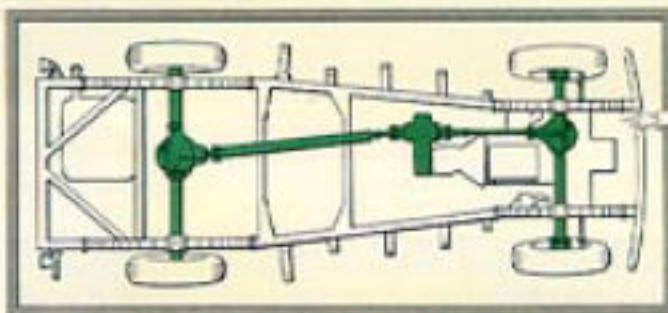
On smooth roads or level ground, you operate a 4-wheel-drive vehicle just like any other car with a standard shift. When necessary, just flick a lever and change over to 4-wheel drive. A special low gear range gives extra pulling power for emergencies, assures you
