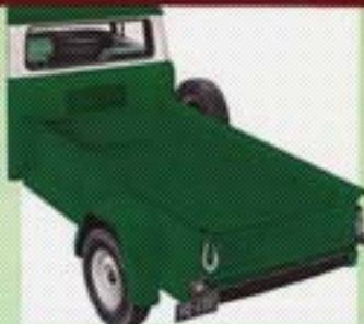
The FC-170 has the greatest cargo area for its length and wheelbase of any truck in its weight class. Here is real capacity to serve you triple . . . 3510 pounds of payload . . . 45 cubic feet of cargo space . . . 9 feet of unobstructed floor length in this big pickup box, on a vehicle which is just over 15 feet long. The rugged box is all-steel construction and is ribbed for easier loading and unloading. Low bed height of only 27 inches gives the FC-170 the lowest loading height in its class.
