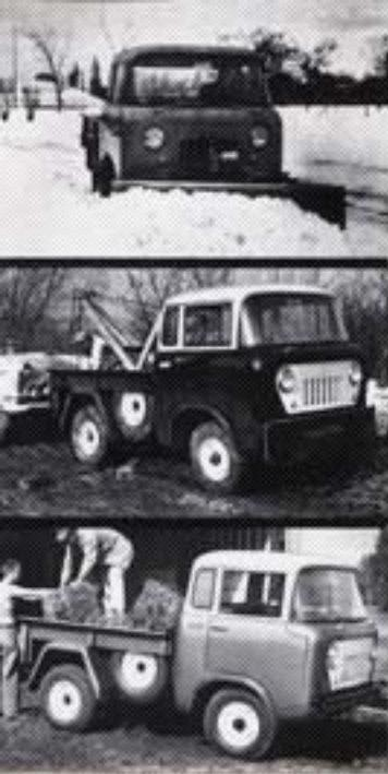
Snow removal is easy with the FC-150 and a power take-off-operated snow plow. "Double-traction" action of 4-wheel drive holds the slipperiest road. Reversible and "V" blade plows come in widths of 6, 7 and 8 feet.
