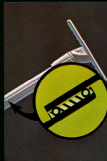
Energy-absorbing steering column
