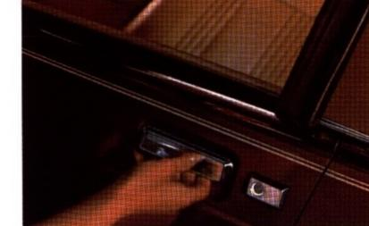
ILLUMINATED ENTRY SYSTEM. When you lift the door handle, a ring of light appears around the keyhole. And, at the same time, the interior lights go on. A great convenience feature.
