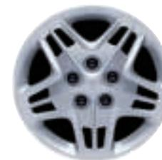
16" steel wheels with a bolt-on cover. Standard on 1SA FWD models.
