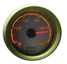
**Battery charge indicator** shows the percentage of the charge remaining on the high-voltage battery.
