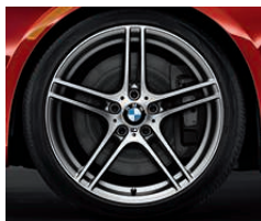
□ 19" M Double Spoke alloy wheels – Style 313 M , 19 x 8.0 front, 225/35R-19, 19 x 9.0 back, 255/30R-19. (Standard on the BMW 335is Coupé.)
