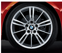
□ 18" M Star Spoke alloy wheels – Style 193 M , 18 x 8.0 front, 225/40R-18, 18 x 8.5 rear, 225/35R-18. (Available on the BMW xDrive 335i Coupé in conjunction with M Sport Package.)
