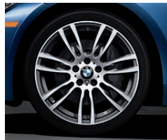
19" Double Spoke alloy wheels - Style 403M, with run-flat performance tires. In front: 19 x 8.0 wheels and 225/40R-19 tires; in back: 19 x 8.5 wheels and 255/35R-19 tires.
