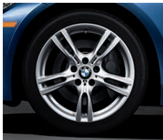
18" Double Spoke alloy wheels - Style 400M, with run-flat performance tires. In front: 18 x 8.0 wheels and 225/45R-18 tires; in back: 18 x 8.5 wheels and 255/40R-18 tires.
