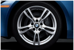
18" M Double Spoke alloy wheels - Style 400M, with 225/45R-18 front and 255/40R-18 rear run-flat performance tires.
