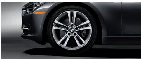
18" Double Spoke alloy wheels - Style 397, with 225/45R-18 run-flat performance tires.
