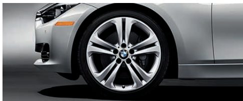
19" Double Spoke alloy wheels - Style 401, with run-flat performance tires. In front: 19 x 8.0 wheels and 225/40R-19 tires; in back: 19 x 8.5 wheels and 255/35R-19 tires. (Only available with the 335i.)
