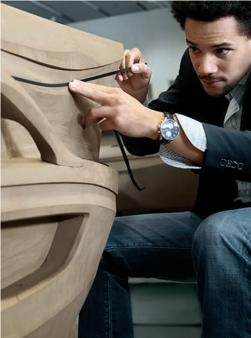
Interior designer Oliver Heilmer checking the lines and dimensions of the body on the clay model.
