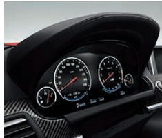
Extended instrument cluster features Black Panel Display with permanently illuminated white surrounds for speedometre and rev counter plus fuel level and oil temperature displays.
