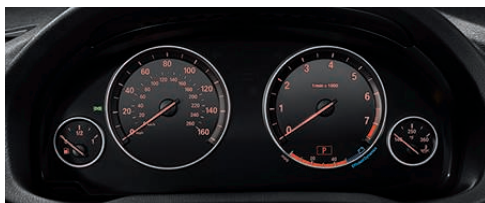
Instrument panel features a red backlit speedometer and tachometer. Centred between the two easy-to-read analog instruments is the on-board computer with liquid crystal display providing additional important driving information.
