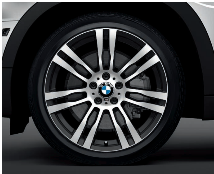
BMW M Double Spoke alloy wheels – Style 333M , 20 x 10.0 front, 275/40R-20, 20 x 11.0 rear, 315/35R-20 (available only with the M Sport Package).
