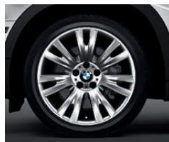
BMW M V Spoke alloy wheels – Style 223M , 19 x 9.0 front, 255/50R-19, 19 x 10.0 rear, 285/45R-19 (available only on the BMW X5 xDrive35i with M Sport Package).
