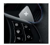
The M Drive function acts as a "memory button" for key driving dynamics, including suspension, stability, steering and throttle sensitivity. Customize these driving dynamics using the iDrive Controller by selecting either Normal (default mode) or Sport mode. In addition, Dynamic Stability Control has three modes: Off, Normal and M Dynamic Mode. Once these settings are saved, just press the M Drive button, and they're recalled for driver convenience.
