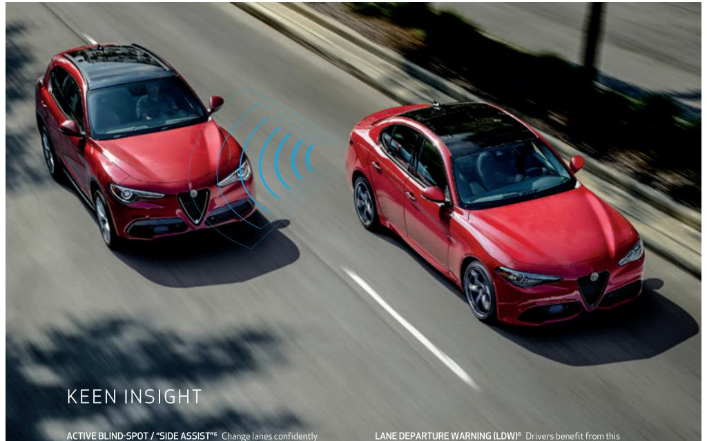
ACTIVE BLIND-SPOT / "SIDE ASSIST" Change lanes confidently or stay right where you are with this available warning system that detects approaching traffic from behind, along with its rate of travel. An LED signal in the corresponding exterior side mirror indicates a vehicle that's too close, while steering-wheel resistance adds another accident-avoidance action.
