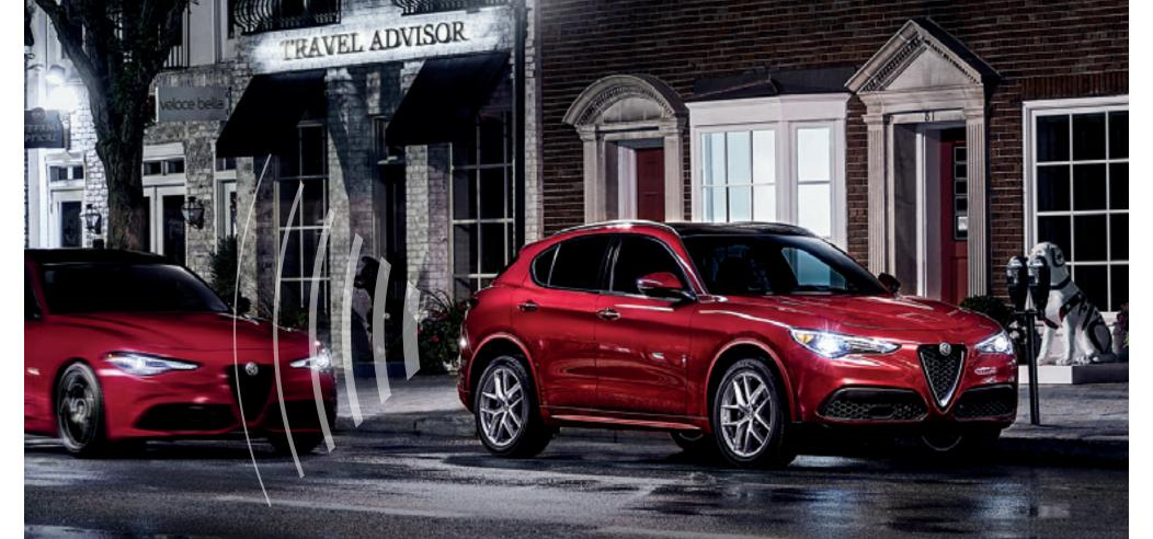
ACTIVE BLIND-SPOT / "SIDE ASSIST"<sup>2</sup> Change lanes confidently or stay right where you are with this warning system that detects approaching traffic from behind, along with its rate of travel. An LED signal in the corresponding exterior side mirror indicates a vehicle that's too close, while steering-wheel resistance adds another accident-avoidance action. Available.
