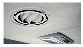
**Rear diffused air vents** let rear passengers diffuse the air flow to a softer, more indirect output.
