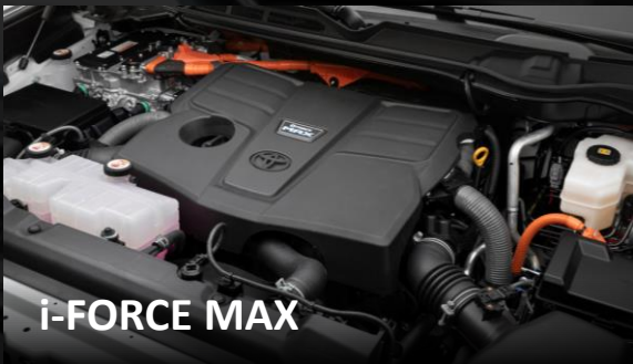
i-FORCE MAX 3.5L Twin-Turbo V6 Hybrid* 437 hp 43 | 583 lb.-ft. of torque Up to 23 mpg comb. (est.) 44 *Available Early 2022.
