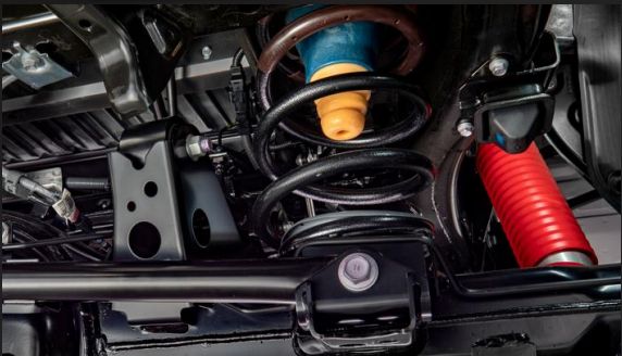
Multi-link rear suspension enhances driving stability and towing capability.
