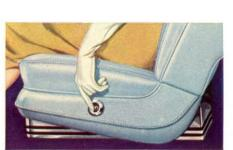
Lincoln Four-Way Power Seat has one switch. Just touch it and the seat moves up or down, backward or forward, until you're in the most comfortable driving position for you. This Lincoln "first" provides a completely individual, customized driving seat—and wonderful comfort. (Standard equipment on Premiere, extra-cost option on Capris.)
