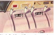
Lincoln Dual-Control Heater combines an underseat heater with a front compartment heater, which can be operated separately to get the desired degree of warmth. A two-speed blower circulates air, defrosts windshield.
