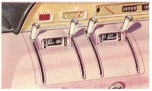
Lincoln Dual-Control Heater combines an underseat heater with a front compartment heater, which can be operated separately to get the desired degree of warmth. A two-speed blower circulates air, defrosts windshield.
