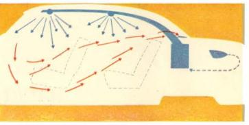
Lincoln Air Conditioning cools, cleans, dehumidifies and circulates up to 258 cubic feet of air per minute—gives you perfect comfort no matter how hot the weather. There are four air inlets, one over each door, controlled by individual louvers.
