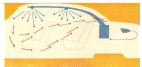
Lincoln Air Conditioning cools, cleans, dehumidifies and circulates up to 258 cubic feet of air per minute—gives you perfect comfort no matter how hot the weather. There are four air inlets, one over each door, controlled by individual louvers.
