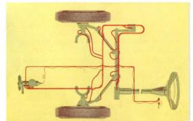
Lincoln Push-Button Lubrication gives you proper lubrication of front-end suspension and steering at just the push of a button. This power-operated system has a reservoir which holds grease for from 250 to 300 lubrications. No matter how dusty the weather, your Lincoln will be properly lubricated, keep that "new car feel" longer. A Lincoln "first," optional at moderate extra cost.
