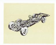
The riding comfort was complemented by the development of the unique Continental Mark II chassis illustrated below. This features a distinctly new type of frame which has side-rails outside the seats, permitting more seating room in a low car, better passenger protection, greater stability and an exceptionally more comfortable ride.
