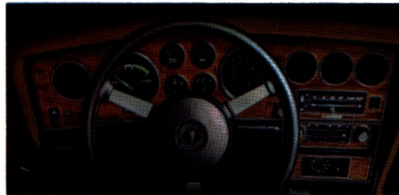
Grand Am instrument panel with standard rally gauges, custom sport wheel and available fuel economy gauge.
