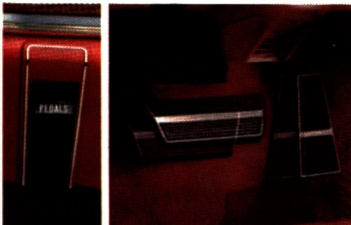
Adjustable pedals you can order. A control on the instrument panel moves the pedals toward you—or away from you—and then locks them into position.
