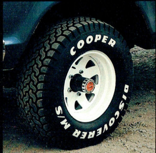
Steel spoke, 15 x 8 wheels and 11 x 15 Cooper Discoverer M/S (mud/snow tread) tyres. Optional at extra cost.
