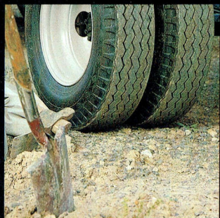
Double rear wheels to assist load capability.
