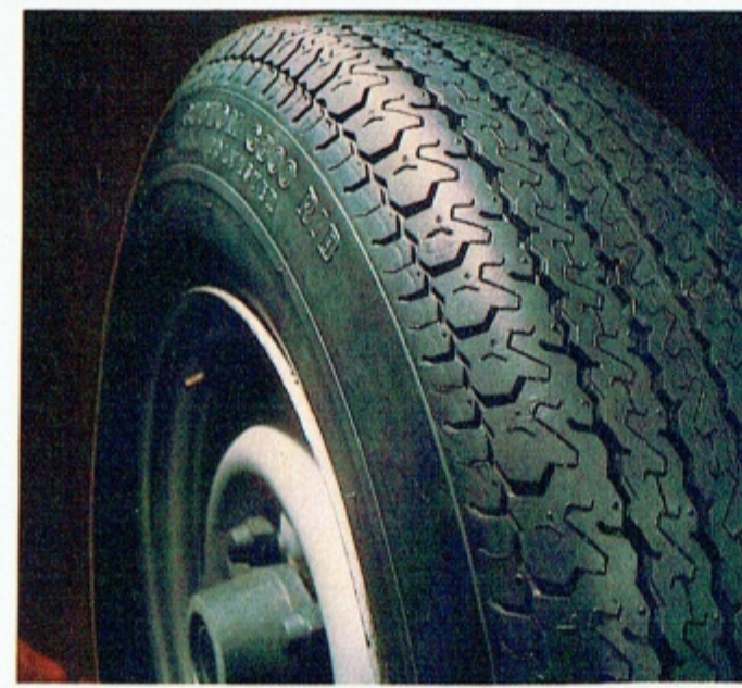
Steel belt radial ply tyres.
