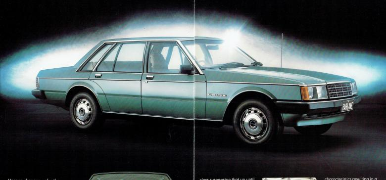
Unseen changes make the difference. The clean contemporary lines of Fairlane may look familiar but underneath there are radical engineering changes. Through the adoption of a Watts Link Rear Suspension System, road holding and ride comfort have been measurably improved, especially over indifferent road surfaces. This system employs trailing arms and the Watts linkage of two transverse rods to control axle location. In combination with progressive rate coil springs, the system provides a world-
