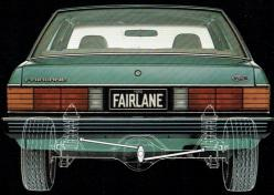
class suspension that up until now has only been available on a small number of imported luxury/sports vehicles. The Watts Link system also delivers improved towing stability by virtue of its more accurate location of the rear axle. A valuable additional benefit is quietness. With less unsprung suspension weight, there is a significant reduction in road generated noise, vibration and harshness.
