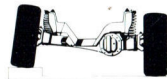
Ford 4WD independent front suspension showing how each wheel operates independently of the other providing a controlled ride.
