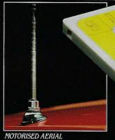
Reduce the risk of vandalism or other aerial damage-with the turn of a switch the radio aerial can be raised or lowered.
