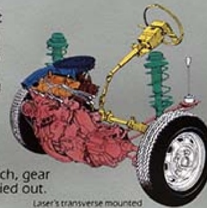
Laser's transverse mounted engine and transmission.
