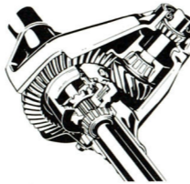
Ford 4WD independent front suspension showing how each wheel operates independently of the other providing a controlled ride.
