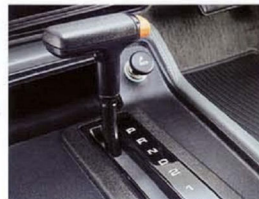
3-speed T-Bar automatic transmission is standard equipment.
