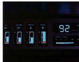
Comprehensive electronic instrumentation with high visibility vacuum fluorescent displays.
