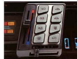
Ventilation, heating and air-conditioning controls are pod-mounted within a finger's reach of the steering wheel.
