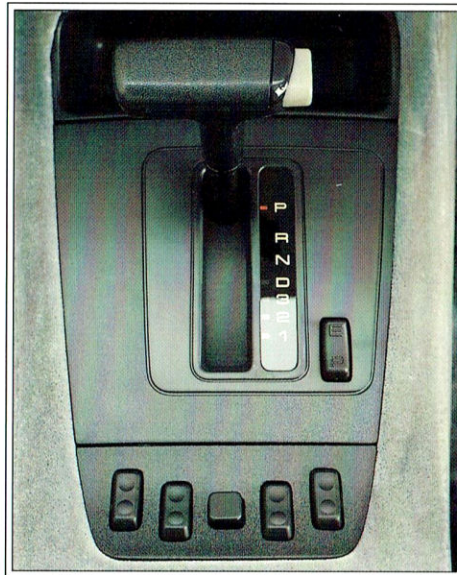
Electronically controlled four speed automatic transmission with electronic power/economy switch.
