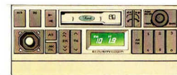
The radio and cassette player is protected by a programmed security code rendering the unit useless to thieves.
