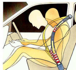
Belt locker device minimises payout of seat belt webbing under extreme conditions.
