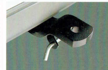
1200 kg rated Towbar. Specially designed for Falcon. Meets Australian Design Rules (ADR62) specifications.
