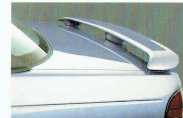
Deck Lid Spoiler. Improves vehicle aerodynamics and adds more style.
