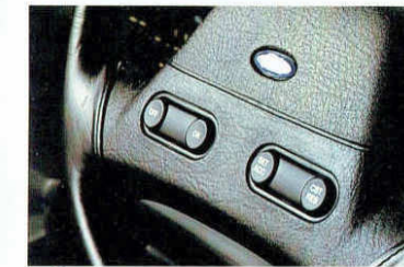
Cruise Control. (Standard on Futura) Helps maintain a constant speed on the open road. Instantly disengages when brakes or clutch are applied.
