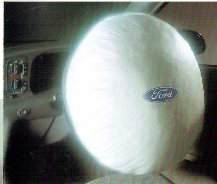
▲ The driver airbag is located behind a panel in the centre of the steering wheel.
