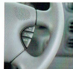
CRUISE CONTROL (Standard on Futura.) Helps maintain a constant speed. Disengages when brakes or clutch are applied.
