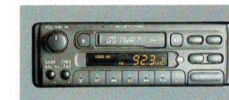
▶ The vehicle's audio system is protected by another Ford anti-theft measure. A special security code renders the unit useless to thieves.
