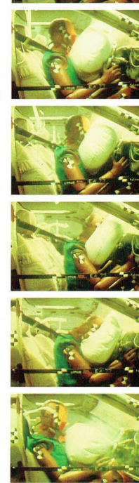
▲ The driver airbag is now standard on every Falcon model. Sensors in the vehicle detect the severity of an impact. If the collision meets the criteria for deployment, the airbag will inflate and be released to help protect the driver. All this occurs in less than one twentieth of a second.
