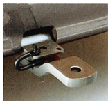
1600 kg TOWBAR* Designed to comply with Australian Design Rule (ADR 62) specification.
