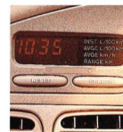
Trip computer calculates fuel and distance data.
