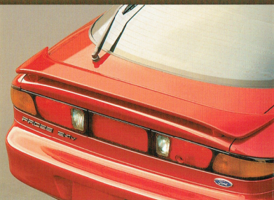
Today's Probe is equipped with a rear spoiler (above) for greater rear wheel traction.
