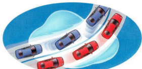
The anti-lock braking system (ABS) is designed to help you maintain steering control in emergency braking situations.
