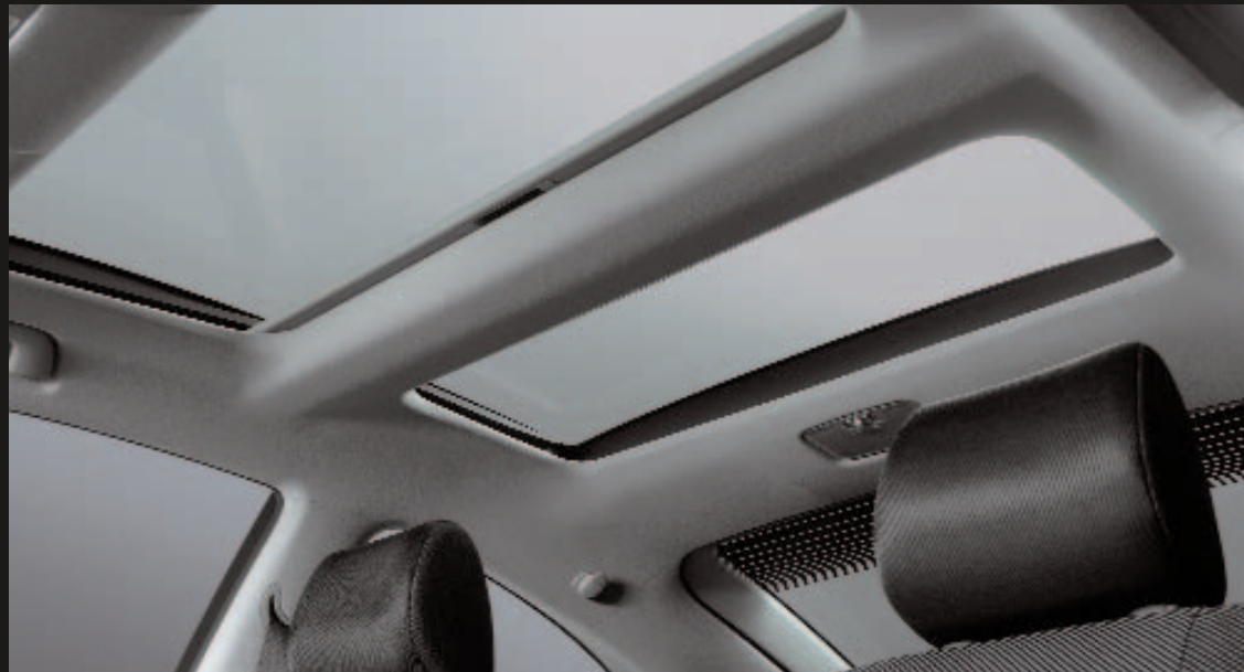
Panorama Moonroof with Power Retractable Front Glass Panel and Dual Manual Sunshades
