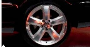
**18" 5-Spoke Aluminum Alloy Multi-Piece Wheel**<sup>1</sup> Finish: titanium silver, high-sheen polish Wheel Size: 7.5J x 18 ET 37 | Tire Size: 225/40 R18 Option for rear axle: Wheel Size: 8.5J x 18 ET 30 | Tire Size: 255/35 R18
