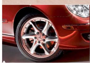
**17" 6-Spoke Aluminum Alloy Multi-Piece Wheel**<sup>1</sup> Finish: sterling silver Wheel Size: 7.5J x 17 ET 36 | Tire Size: 225/45 R17 Option for rear axle:<sup>1</sup> Wheel Size: 8.5J x 17 ET 30 | Tire Size: 245/40 R17
