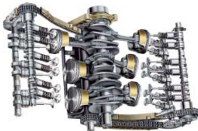
Main rotating assembly and valve gear
