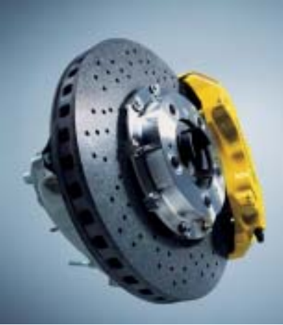
Porsche Ceramic Composite Brake (PCCB)
