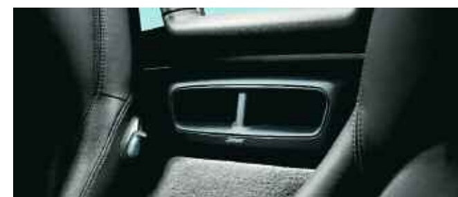
Active subwoofer with 2 x 13.0-cm low-range speakers and 2 x 6.5-cm mid/high-range speakers
