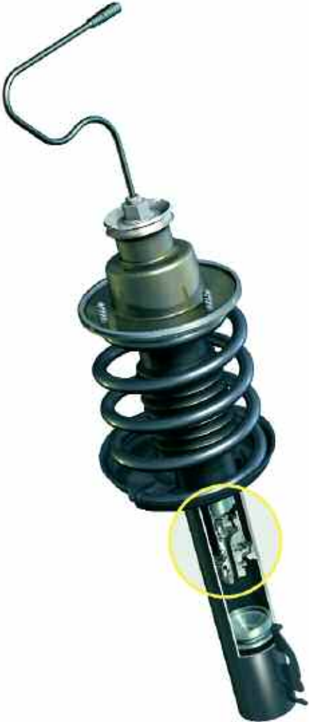
Rebound in 'Normal' mode – damper piston with bypass valve open
