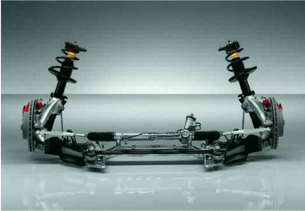
Front axle with McPherson struts and lateral control arms (Cayman S)
