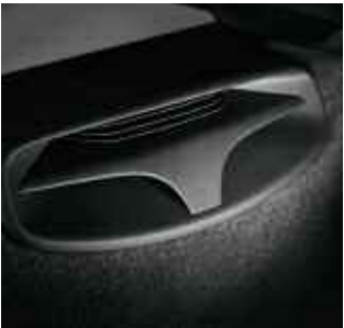
Active subwoofer with 10.2-cm x 15.3-cm low-range speaker in passenger footwell
