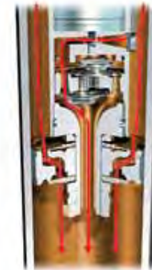
Rebound in 'Normal' mode – damper piston with bypass valve open
