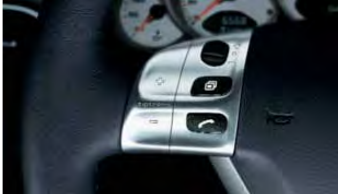
Tiptronic S control on steering wheel
