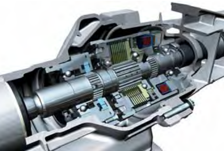
Electronically controlled multi-plate clutch
