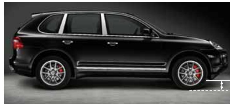
Normal Level: 215 mm Cayenne GTS: 195 mm
