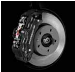
Cayenne: standard front brake with 330-mm disc
