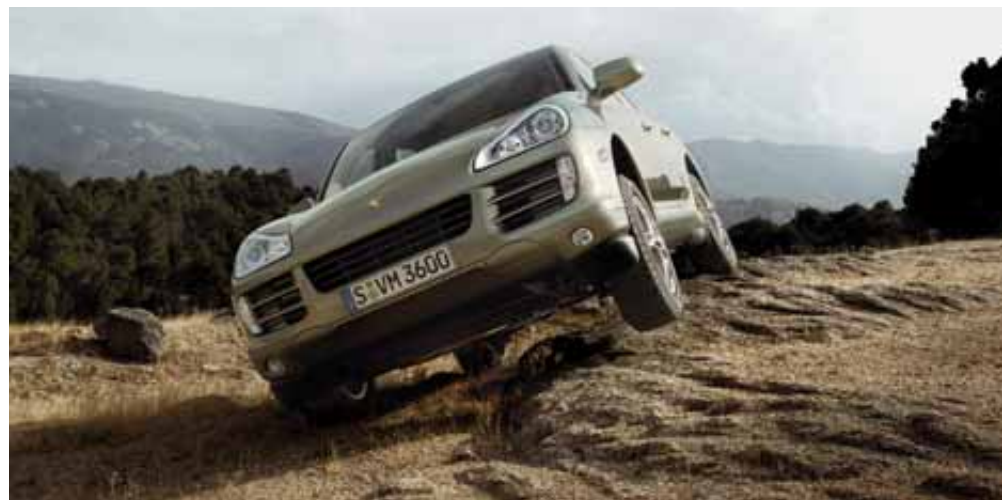
PDCC in on-road mode: reduced wheel articulation
