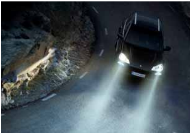
Cornering light function on Bi-Xenon headlights
