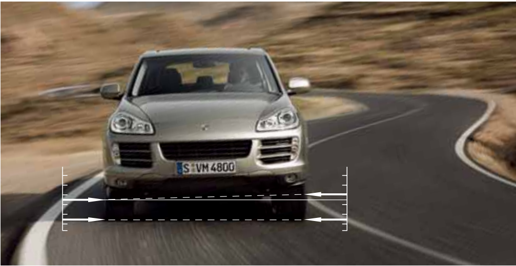
High-speed cornering without PDCC
