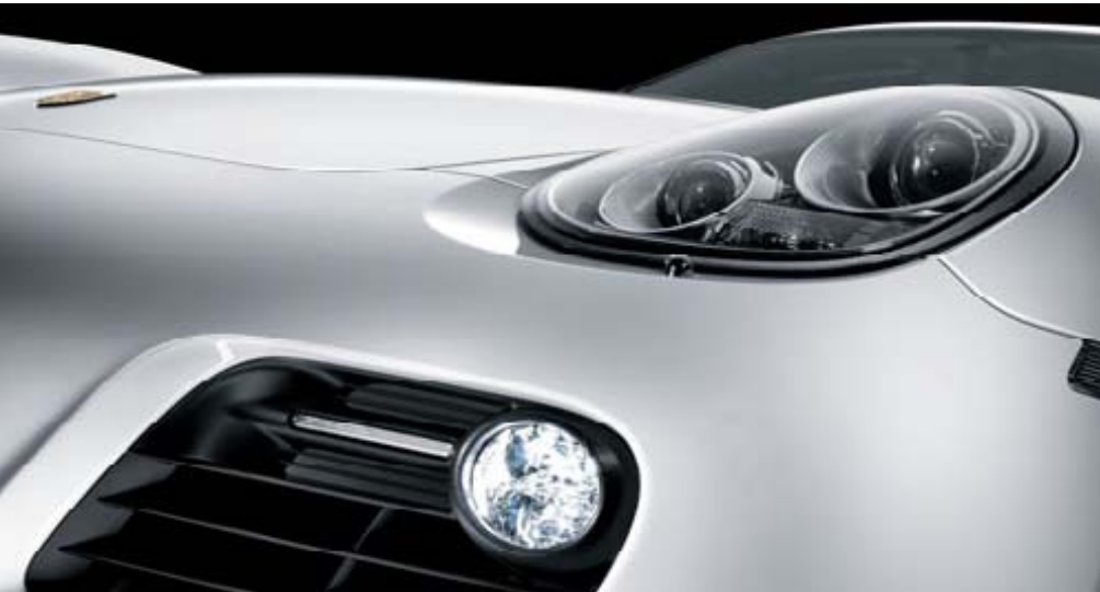
Bi-Xenon headlights with dynamic cornering lights and LED daytime running lights
