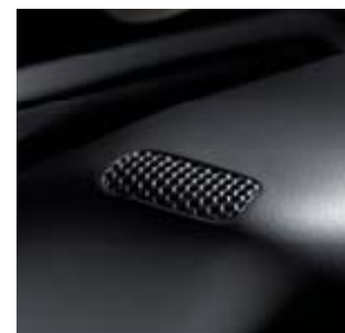
Microphone for AudioPilot® on the steering column
