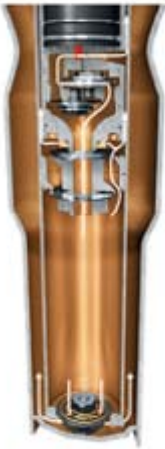
Rebound in 'Normal' mode – working piston and bypass, sporty-comfortable tuning
