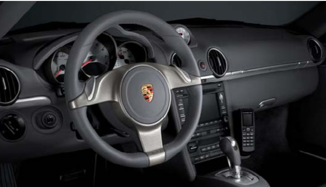
Sports steering wheel with gear shift switches for PDK
