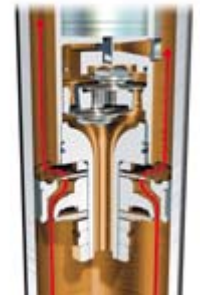
Compression in 'Sport' mode – working piston only, sporty-hard tuning
