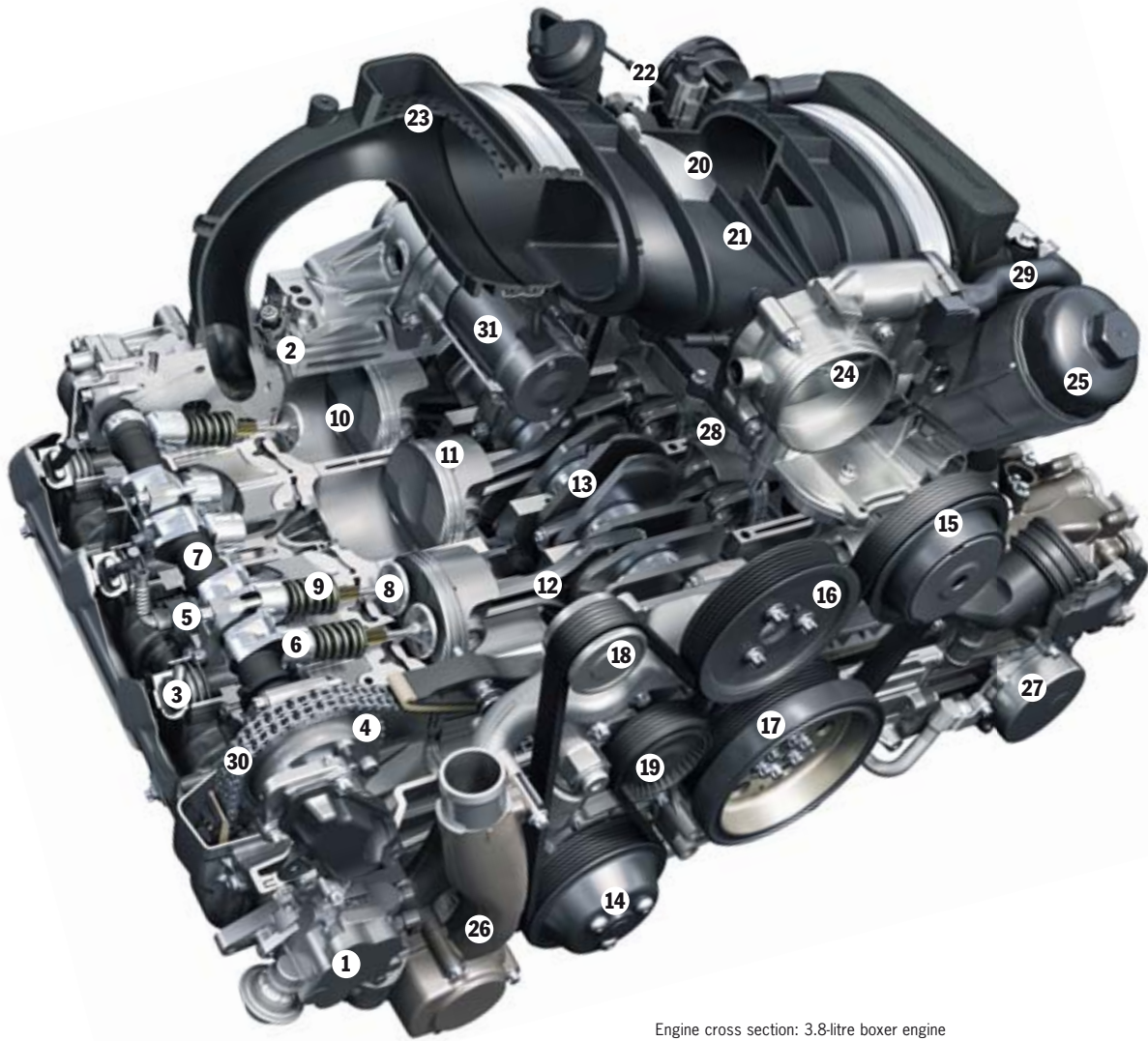
Engine cross section: 3.8-litre boxer engine
