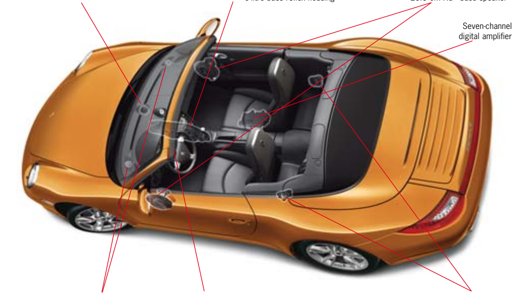
Subwoofer 10.2 cm x 15.3 cm in a 6-litre bass reflex housing
