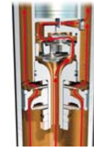
Compression in 'Normal' mode – working piston and bypass, sporty-comfortable tuning
