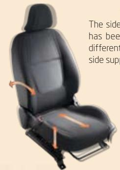
The side bolster of the driver seat has been enlarged, and features different firmness levels for better side support.
