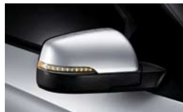
Outside mirrors with side repeaters The outside mirrors now feature LED side repeaters, providing not only a more modern look, but also more visibility to oncoming traffic when turning for added safety.
