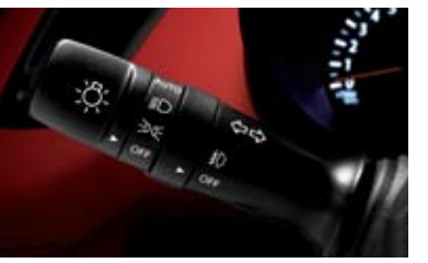
Auto light control Auto light control saves you having to operate the lights manually, the headlamps and rear lights automatically turning on and off according to the light conditions.
