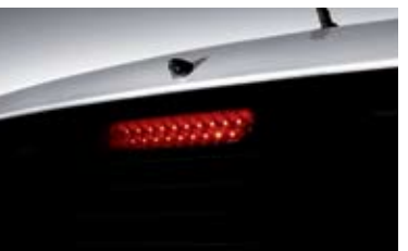
Rear spoiler / High mount stop lamp The rear spoiler flows from the roofline, aiding aerodynamics and sheltering the high mounted stop light - a valuable safety feature that ensures your braking intentions are seen.
