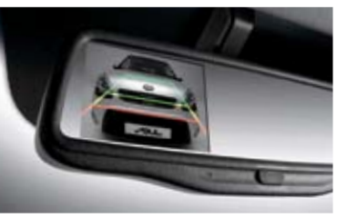
Rear display / ECM room mirror The rear view mirror uses an inconspicuous 130-degree rear-mounted camera to determine risk factors behind you when reversing. The electrochromic mirror (ECM) function will also dim any light glare from headlamps behind you. (Standard)
